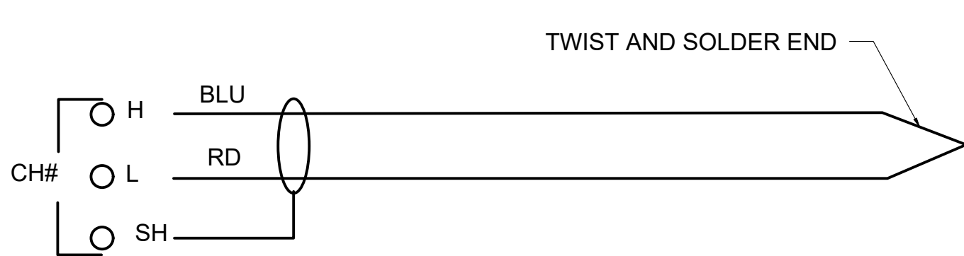
THERMOCOUPLE EXTENSION CABLE WIRING DIAGRAM
